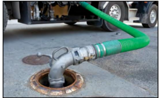
**CONSTRUCTION:** Polyurethane tube, smooth bore with embedded SΩ ground wire in the hose wall with a sturdy clockwise PVC helix, one braid of high tensile polyester yarn reinforcement.
