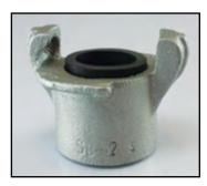
THREADED POT ENDS do not fit the hose, but rather are threaded (NPT or NPS) onto the sandblast pot. Once properly threaded to the discharge pipe on the pot, the 2 lug crowfoot design can now be connected to the 2 lug crowfoot design of the hose end. Now the pot can supply mix to the operator by way of the hose to the sandblast nozzle.
