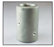
**NOZZLE HOLDERS** are sleeve type couplings, secured to the hose with wood screws and have the same features as the sandblast hose end. The exception is that the end of the nozzle holder is NPT threaded to accept the sandblasting nozzle.
