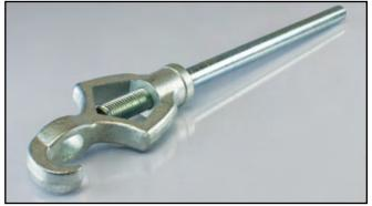
Lighter in weight than the HYD-1 with the same adjustable features. Fits 1-3/4" pentagonal nuts. The head will operate hydrant cap and adapter pin or rocker lugs. Handle is plated.
