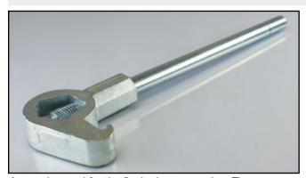
A complete tool for the fire hydrant operation. The pentagonal nut head is adjustable to fit hydrant valves to 1-3/4" for on/off operation. The head also operates pin lug or rocker lug connections from 1-1/2" to 6"
