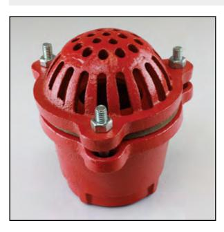
Foot valves are used on the submersed end of the water suction hose to prevent the pump from losing it's prime when shut down. The foot valve stops the water from draining by a closing leather flapper gate. Each valve has a built in strainer that prevents debris from entering during operation. All sizes have NPS threads and complete valves are painted red.
