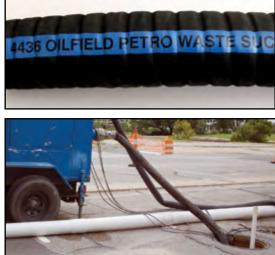
**CONSTRUCTION:** Tube is an NBR/SBR blend, black and smooth, oil resistant. Cover is an NBR/ PVC blend, black, flat corrugated w/ cloth impression, oil, abrasion, weather and ozone resistant. Reinforcement is a high tensile cord with a dual steel wire helix.
