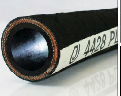
CONSTRUCTION: Tube is NR/SBR blend. Cover is a NR/SBR blend, pin-pricked. Reinforcement is four plies of synthetic textile with a static wire.
