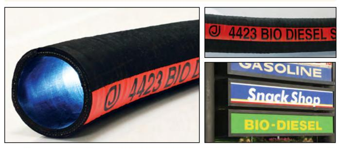
**CONSTRUCTION:** Tube is ultra-high molecular weight polyethylene (UHMWPE). Cover is CR, smooth and black. Reinforcement is a two-ply synthetic
