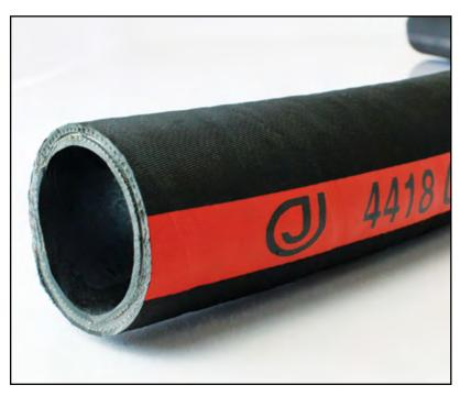
**CONSTRUCTION:** Tube and cover are EPDM. Reinforcement is a two-ply synthetic fabric with a wire helix.
