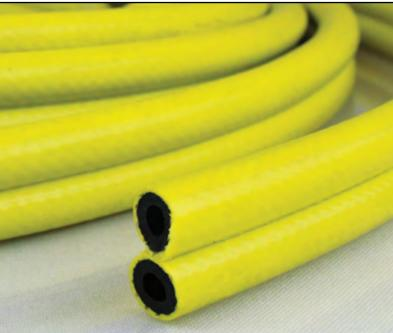
**CONSTRUCTION:** Tube and cover are TPR (NBR/PVC). Cover is yellow. Reinforcement is two spirals, synthetic fabric.
