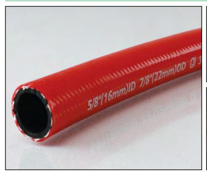
**CONSTRUCTION:** Tube and cover are PVC, smooth, medium oil resistance, ARPM Class C. Cover is red. Reinforcement is one braid, synthetic material.
