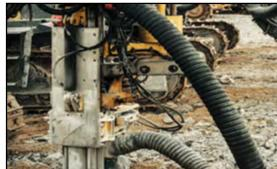
**CONSTRUCTION:** Abrasion resistant SBR tube and cover
